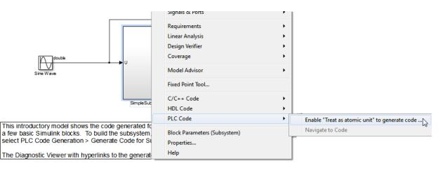
This command opens the block parameter dialog box so that you can select the **Treat as atomic unit** check box.
