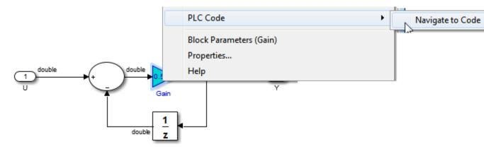
**2** Selecting **Navigate to Code** activates the HTML code generation report. The following figure shows the result of tracing the Gain block within the subsystem.
